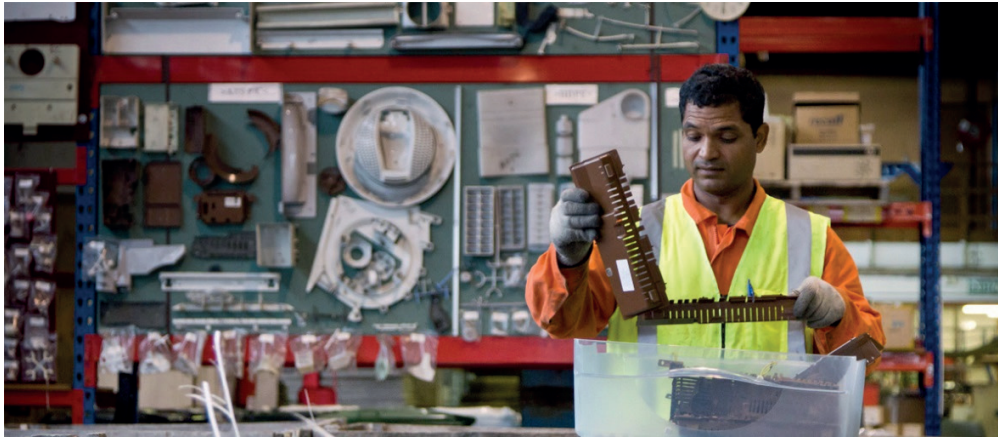
Figure 2: Fisher & Paykel Appliances employee taking apart their products at the end of its useful life
