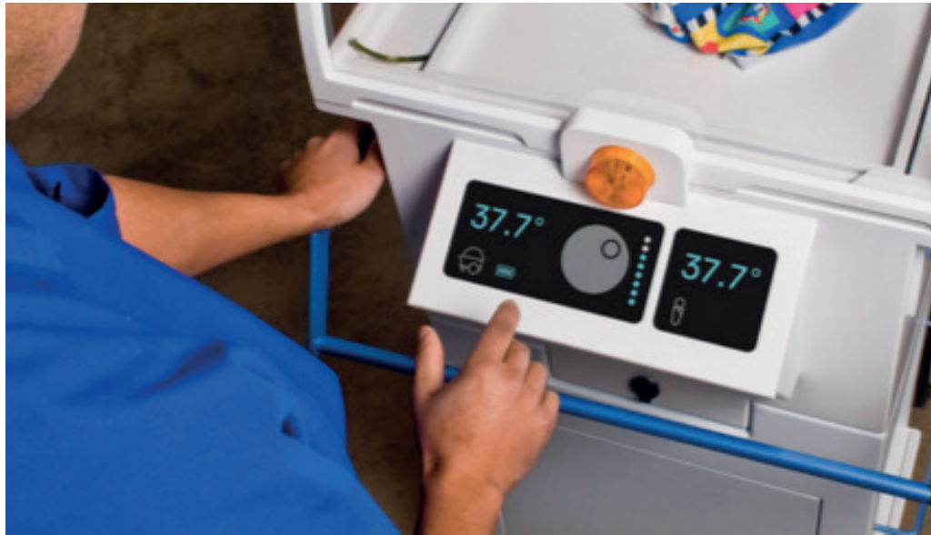
Figure 7: The user interface provides access to the controls of the NeoNurture, enabling the user to set variables including temperature and time
